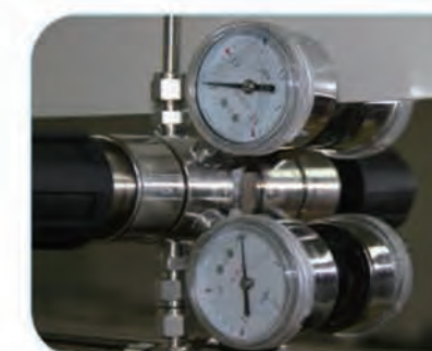
First Stage Regulator Max Output: 25MP-250KG Min Input: 0.1MP-1KG
